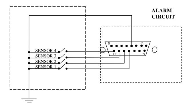
There are four alarm inputs for each camera. Please connect the alarm input in the same sequence as the cameras input.
